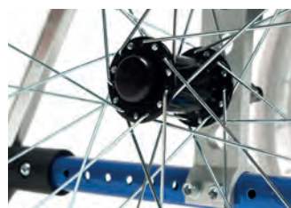
Quick-release wheels for fast disassembly during transport
