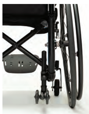
Camber adjustment of the rear wheels
