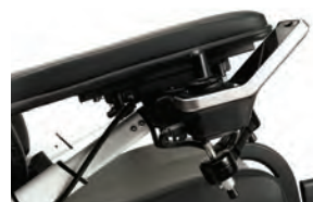
S53Z Drop swing away controller for easy table access
