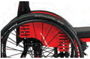
B82-S or B82-C fixed adjustable fixed clothing protectors, in aluminum or carbon
