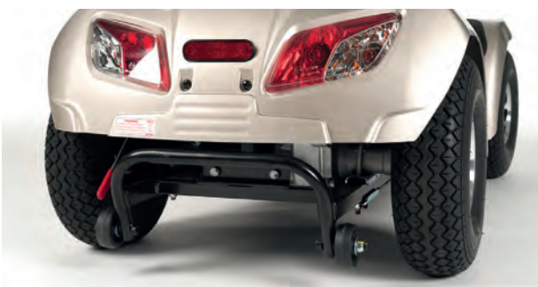
Anti-tipping, front and rear lights and reflectors for optimal safety when driving in the dark.
