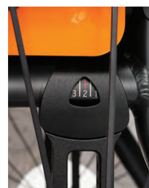
Adjusting the position of the rear wheels
