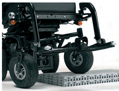
Rotating axle to allow constant ground contact on all the wheels
