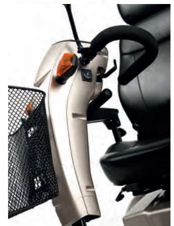
Angle adjustable steering column for more personal driving comfort
